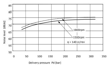
Noise level measured in an anechoic chamber where distance from microphone to pump is 1 metre. Measurement accuracy +/- 2 dB(A)
