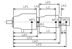
MPX = mass of pump [kg] LPX = length of pump [mm] Lx = distance of CofG from pump mounting face [mm] MAX = mass of adaptor kit [kg] LAX = width of adaptor kit [mm]
