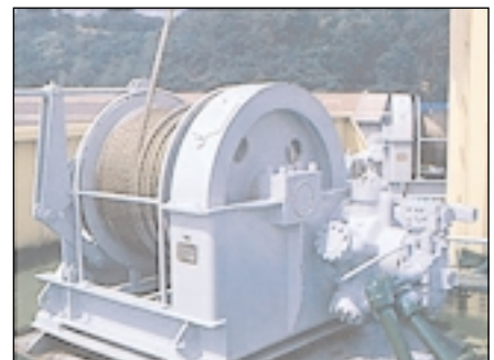
Cargo Winch Pump Used: K3VG180
