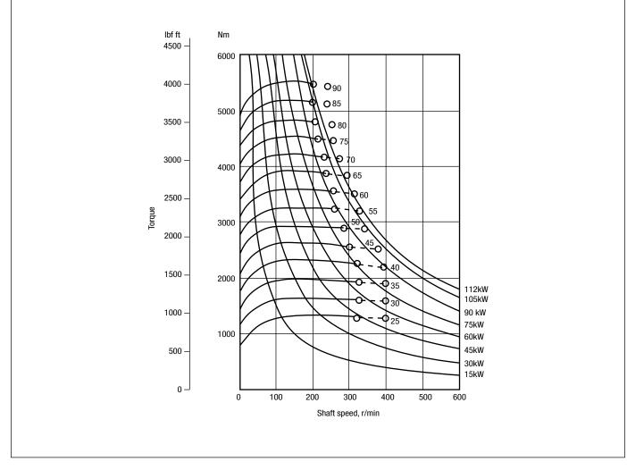
The torque curves indicate, for each displacement, the maximum output torque of the motor with an inlet pressure of 250 bar (3626 psi) and zero output pressure. High return line pressures will reduce the torque for any given pressure differential.
